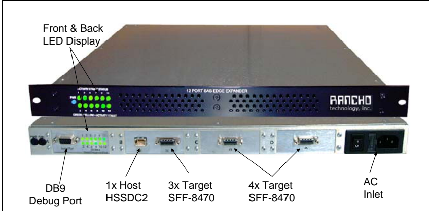
Figure 4: Data connector descriptions. Green = Activity, Yellow = Fault
